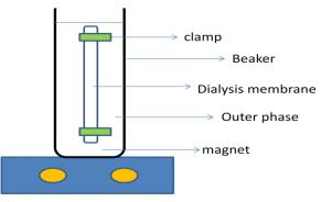
Figure 2.1. Schematic representation of in vitro release experimental system
