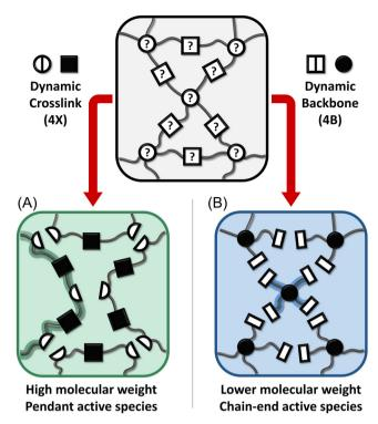
**FIGURE 6** (A). A schematic of the higher molecular weight, lower relative mobility pendant active species formed by the cleavage of a disulfide in a material with only dynamic crosslinks (**4X**); (B). A schematic of the lower molecular weight, higher relative mobility chain-end active species formed by the cleavage of a disulfide in a material with only a dynamic backbone (**4B**).
