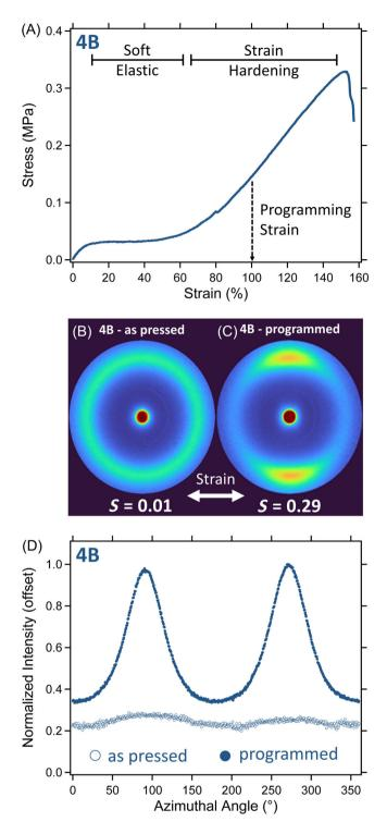
**FIGURE 4** (A). Stress-strain profile of an as pressed sample of **4B**; (B). 2D WAXS image of an as pressed film of **4B**; (C). 2D WAXS image of an aligned programmed film of **4B**; (D). Plots of normalized intensity as a function of angle for both an as pressed and programmed aligned film of **4B**.
