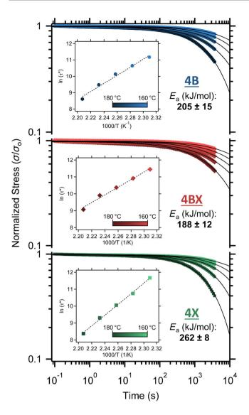
**FIGURE 5** Temperature dependent stress relaxation curves for dynamic LCEs fitted to stretched exponential functions, with  $\tau^*$  values determined by the fit. (Inset) Arrhenius curves demonstrating the linear relationship between ln ( $\tau^*$ ) and temperature for a given sample. Errors for activation energies are derived from the linear fit of the data.
