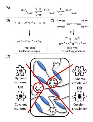
**FIGURE 1** (A). Dynamic exchange of disulfide bonds; (B). Radical initiated reaction mechanism for a dialkene monomer with two thiols forming a linear backbone linkage; (C). Radical initiated reaction mechanism for a dialkyne crosslinker with four thiols forming a crosslink; (D). Schematic depicting the modular nature of this dynamic LCE system that allows for selective disulfide placement in backbone linkages, crosslinks, or both.
