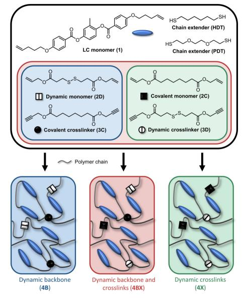
FIGURE 2 Component and network designs for a modular disulfide containing LCE network that allows for selective disulfide placement in backbone linkages, crosslinks, and a system containing both.
